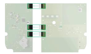
Please note: the board contacts should be plugged into the bottom row of the connector (closest to the board). When connected correctly, the boards are on the same level.
